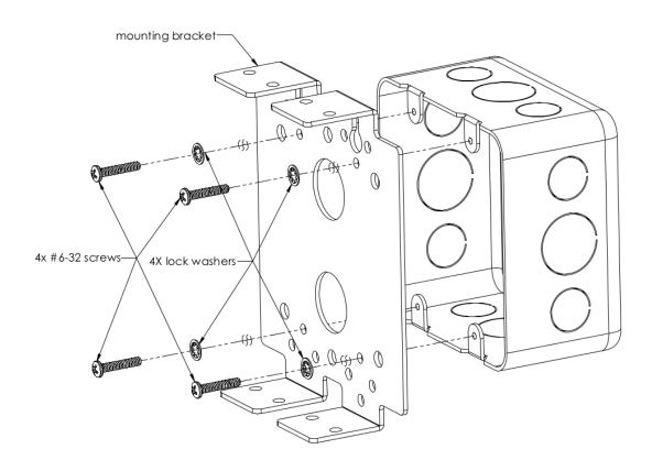
Mount each included bracket to the front of a standard two-gang electrical backbox (preferred), using (4) included #6-32 screws and lock washers per bracket.
