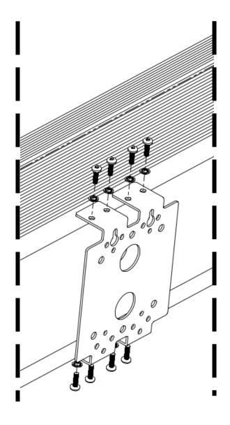
Attach IP Display to brackets using included (8) #8-32 screws and washers per bracket.
