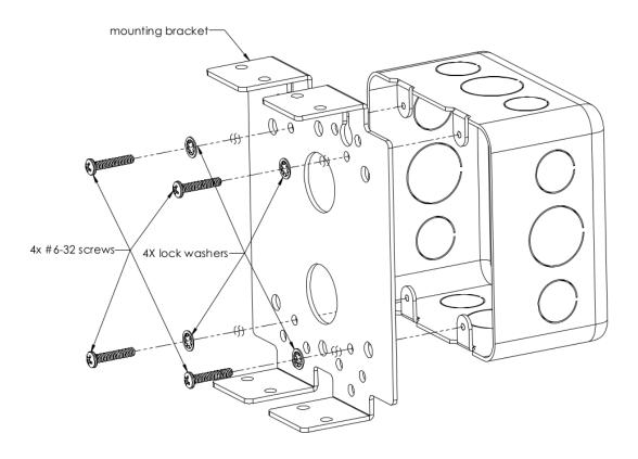
Mount each included bracket to the front of a standard two-gang electrical backbox (preferred), using (4) included #6-32 screws and lock washers per bracket.
