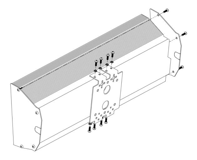
Attach speaker to bracket using included (8) #8-32 screws and washers.
