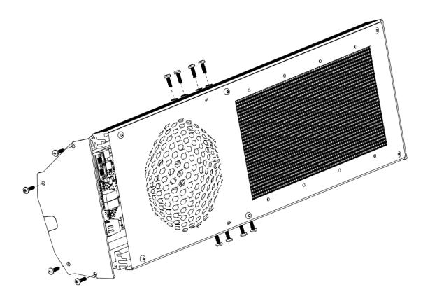
Cable access is available through rear opening or side panel knockout.
