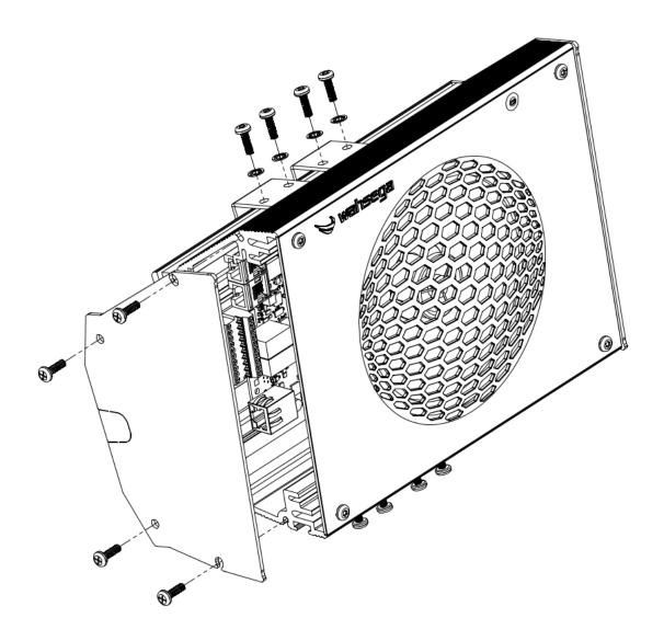
Cable access is available through rear opening or side panel knockout.
