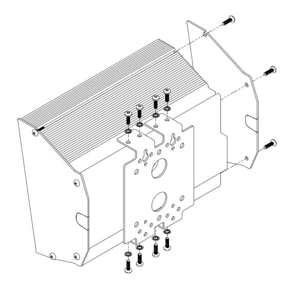
Attach speaker to bracket using included (8) #8-32 screws and washers.
