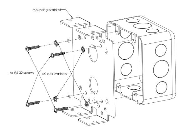
Mount included bracket to the front of a standard two-gang electrical backbox (preferred), using (4) included #6-32 screws and lock washers.
