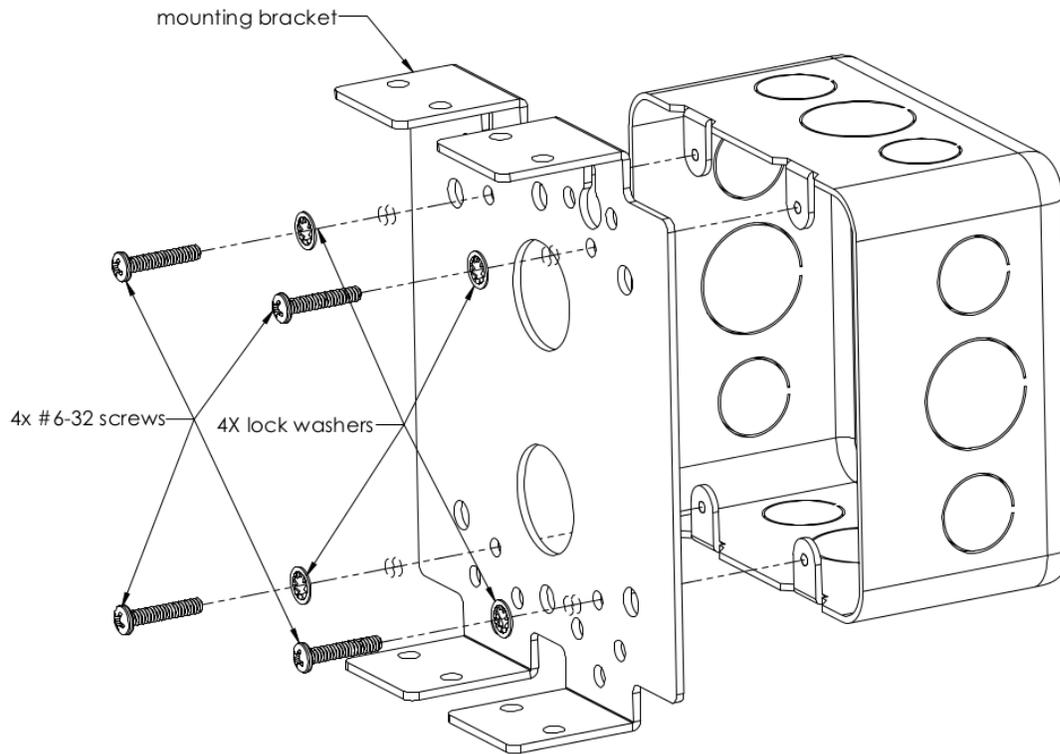
Mount included bracket to the front of a standard two-gang electrical backbox (preferred), using (4) included #6-32 screws and lock washers.
