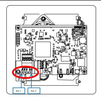
As a "reset to factory defaults" function, two pins on the 7-pin connector can be jumpered together using a standard 2mm electrical jumper. When the intercom boots up, it will check to see if these pins are jumpered, and if so, it will perform a "factory reset". Which pins are jumpered together determines the type of factory reset performed:
