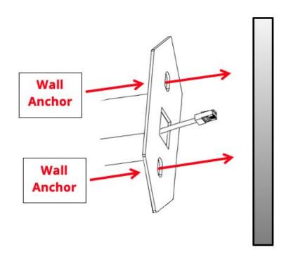
Affix mounting bracket to a solid, vertical wall surface using two bolts and anchors appropriate for the wall surface.
