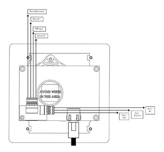
Note: Ethernet cable can ONLY be installed in the orientation shown.
