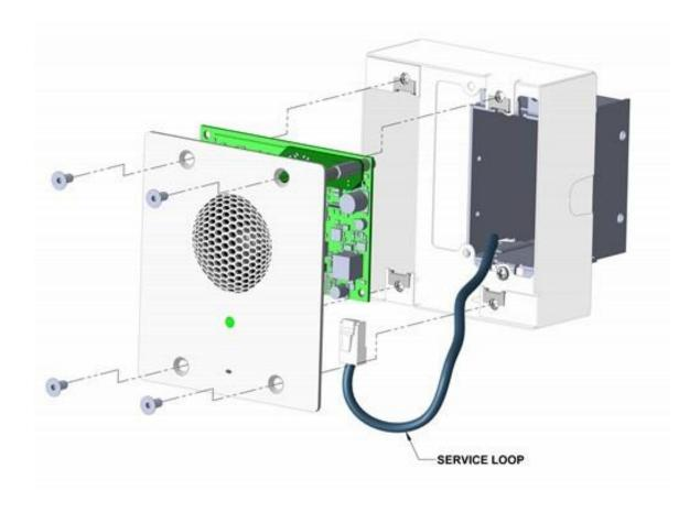
Before installing the faceplate, be sure to locate and note the intercom's MAC address, which is printed on a white sticker on the rear of the circuit board.
